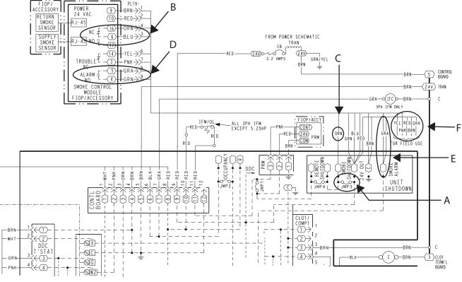
Fig. 23 - Typical Smoke Detector System Wiring
